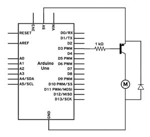
A key point to remember while using PNP transistors with Arduino is that the maximum voltage on the emitter is 5 V, so the motor will never receive more than 5 V. If we use an external power supply for the motor, the base will have a voltage higher than 5 V and will burn the Arduino. One possible solution, which is quite complicated, has been shown here:
