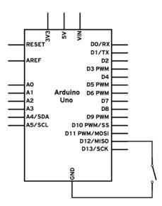
Here is a simple way of wiring the button:
