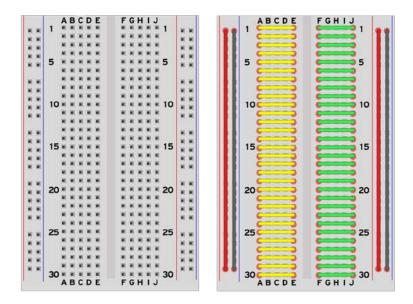
On the left we have a simple breadboard; on the right, we have the same breadboard with the internal connections shown. At the bottom and the top of the board we can see letters. If we follow, we can see that, on each row, the letters **A**, **B**, **C**, **D**, and **E** are interconnected, as shown by the yellow wire.
