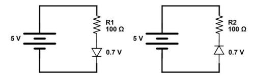
However, even when a diode allows current to pass, it drops the voltage. For a typical value, it drops the voltage by 0.7 V. Let's try and apply Ohm's law to the left circuit again. If the diode drops the voltage by 0.7 V, it means we have 4.3 V across the resistor. This will result in:
