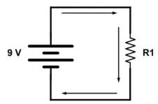
Resistance is the measure of the property of a material to oppose current flow. It's measured in ohms, symbolized by the Greek letter  $\Omega$ . The resistor is the component that uses its internal resistance to restrict current flow. This is the schematic symbol, and next to it, a normal resistor:
