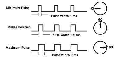
Remember that using the Servo library automatically disables PWM functionality on PWM pins 9 and 10 on the Arduino UNO and similar boards.
