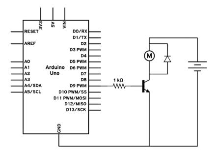
Here is one way of hooking up the motor and the transistor on a breadboard:
