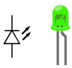
They come in a variety of colors and power ratings. A typical 3-mm green LED will consume around 20 mA and will cause a 1.9 V drop across it. A diode doesn't restrict the amount of current through it, so we should always connect a resistor in series with a diode or LED. In the following schematic, we have a 20 mA LED that causes a 1.9 V drop. Let's try to calculate the perfect resistance for it:
